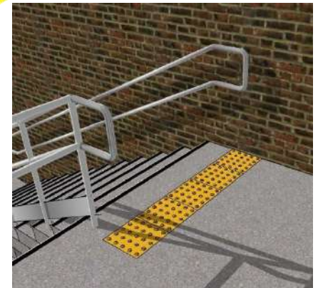
WARNING INDICATORS AT STAIRCASE
